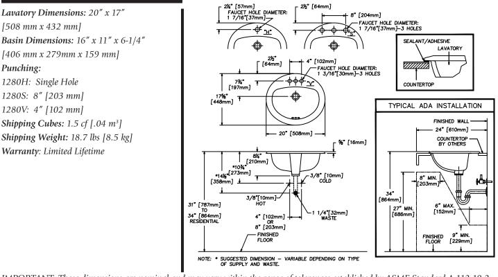
IMPORTANT: These dimensions are nominal and may vary within the range of tolerances established by ASME Standard A 112.19.2
