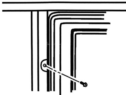
**NOTE:** You must drill pilot holes in cabinet to prevent splitting the wood before installing screws.
