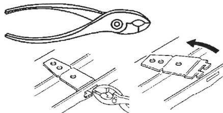
2. Push bracket into slot on the side of dishwasher, and bend tab in towards the side of the dishwasher so that it keeps the bracket in place. Repeat this step on the opposite side of the dishwasher.
