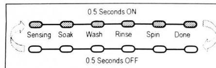
Figure 2 - Status LEDs flashing ON and OFF
